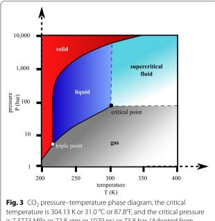
temperature is 304.13 K or 31.0 °C or 87.8°F, and the critical pressure is 7.3773 MPa or 72.8 atm or 1070 psi or 73.8 bar. (Adopted from Wikimedia commons URL: https://upload.wikimedia.org/wikipedia/ commons/1/13/Carbon\_dioxide\_pressure-temperature\_phase\_diagr am.svg)
